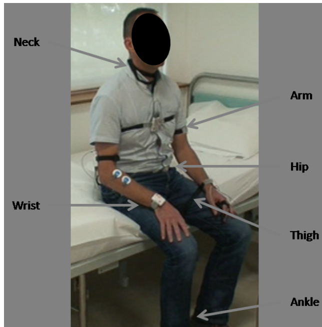
Figure 1: Shimmer3 module positions.
