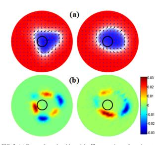
FIG. 2. (a) Frames from the video of the FL magnetic configuration at zero field and  $J = 2 \times 10^6$  A/cm<sup>2</sup> and (b) corresponding topological density (Multimedia view) [URL: http://dx.doi.org/10.1063/1.4867747.3] [URL: http://dx.doi.org/10.1063/1.4867747.4].
