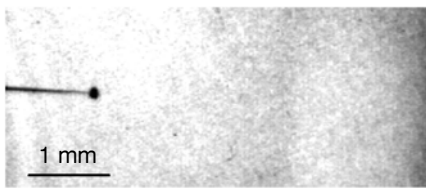
Fig. 2 “1 st mode” slow positive streamer in BT ( V = 10 kV).
