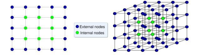
Figure 2: Topological active net and topological active volume structure representation.
