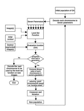
Figure 11: Main workflow diagram for [196].
