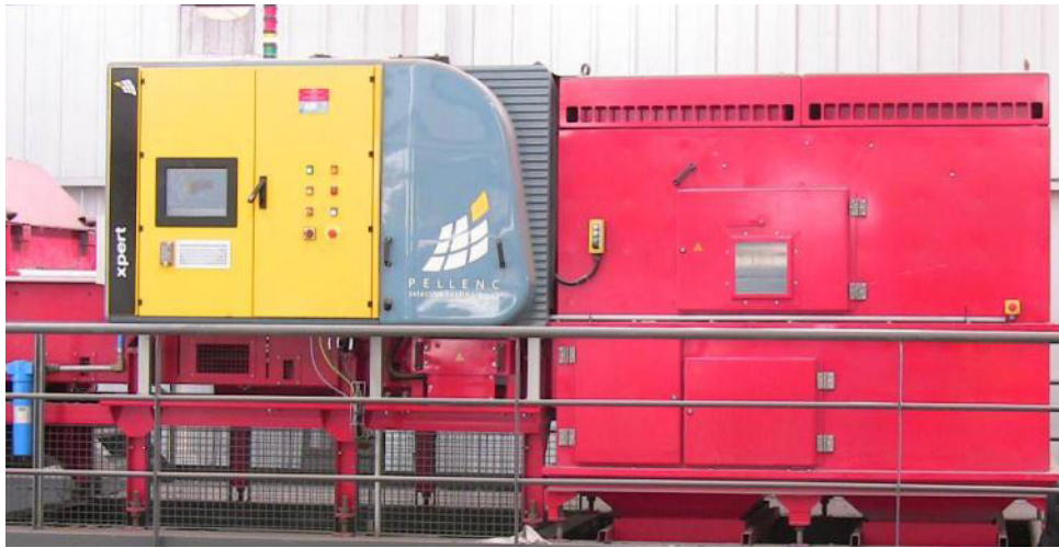
FIGURE 11 : Industrial sorting machine Xpert (PELLENC ST)
