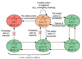
Fig. 8. State diagram illustrating all safety states including the interlock
