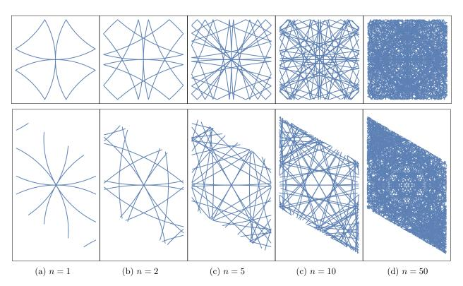
FIG. 1: (color online) Isofrequency lines for a two-dimensional homogeneous medium artificially discretized on a square (top) and triangular (bottom) lattices. The band index is labeled by n. The plots depict the isofrequency lines contained in the FBZ of the lattice and can be periodically replicated in all directions. A mathematical definition of the folding operation is given in Eq. (34).
