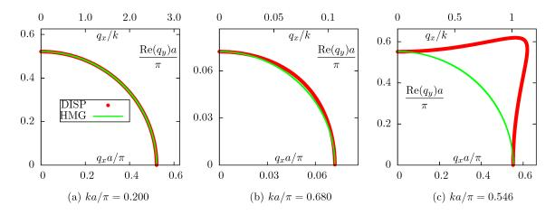
FIG. 5: (color online) Purely real parts of the isofrequency contours shown in Fig. 4. The lines marked 'HMG' are ideal circles.
