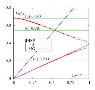
FIG. 3: (color online) Dispersion diagram for the square lattice of hollow cylinders. Frequency is scanned from zero to slightly above the second  $\Gamma$ -point. The variable  $ka/\pi = \omega a/\pi c = 2a/\lambda$  is the dimensionless frequency. The line labeled LL is the light line and the line labeled MG gives the Maxwell-Garnett approximation to the dispersion curve. Thin horizontal lines mark the frequencies at which further simulations have been performed.
