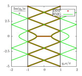
FIG. 9: (color online) An expanded view of  $\text{Im}(q_y)$  as a function of  $q_x$  for  $ka/\pi = 0.200$  [Case (a)]. Here several 'reflected' segments of the isofrequency line are shown. These segments are obtained by folding the corresponding isofrequency line for an infinite homogeneous medium into the FBZ of the triangular lattice according to (38). The analytical lines outside the FBZ (shown by the two vertical lines) are not the actual solutions and are shown only to guide the eye.
