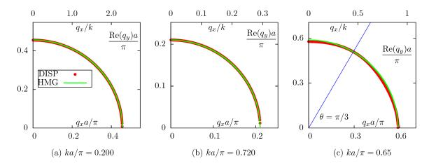
FIG. 10: (color online) Same as in Fig. 5 but for the triangular lattice. Distortions of the quasi-circular lobes are consistent with  $C_6$  symmetry. The straight line in panel (c) makes the  $\pi/3$  angle with the horizontal axis.
