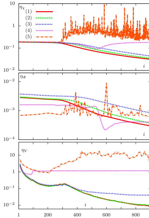
**Figure 7.** Convergence data for the large target. The different curves correspond to different contrast  $\chi_0$  as follows:  $\chi_0 = 0.002$  (1),  $\chi_0 = 0.02$  (2),  $\chi_0 = 0.2$  (3),  $\chi_0 = 1$  (4) and  $\chi_0 = 2$  (5).
