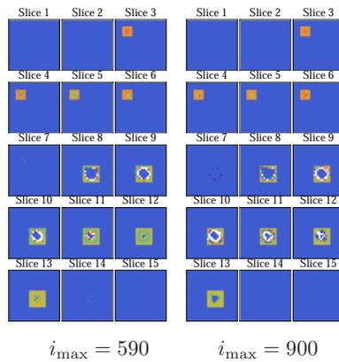
**Figure 8.** Comparison of the reconstructions of the large target with  $\chi_0 = 1$  (Case 4 in Fig. 7) for different numbers of iterations  $i_{\max}$ , as labeled. Reconstruction with  $i_{\max} = 490$  is marginally better than the reconstruction with  $i_{\max} = 900$ .
