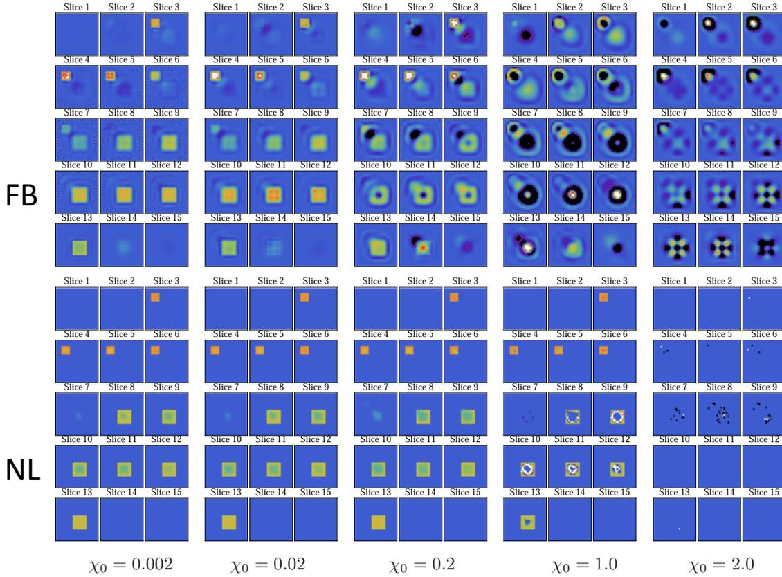
**Figure 6.** Same as in Fig. 2, but for the large target, near-field zone source/detector arrangement (see Sec. 3.4), and a somewhat different set of contrasts  $\chi_0$ . Utilization of first Rytov approximation for linearized reconstruction does not provide any improvements over first Born approximation, and the corresponding results are not shown in this figure.
