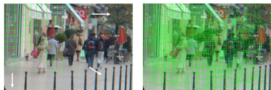
Figure 1: Sliding-window illustration (left) and randomly sampled 1% of all windows (right) on a 769 \times 516 sample image taken from the public INRIA person dataset.
