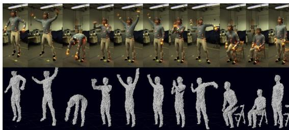
Figure 2: Snapshots from all the actions available in the Berkeley MHAD displayed together with the corresponding point clouds obtained from the Kinect depth data. Actions (from left to right): *jumping*, *jumping jacks*, *bending*, *punching*, *waving two hands*, *waving one hand*, *clapping*, *throwing*, *sit down/stand up*, *sit down*, *stand up*.
