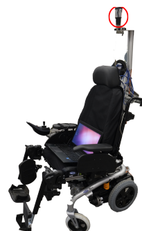
Figure 1: The wheelchair equipped with the omnidirectional camera, on top of it surrounded by the red ellipse.
