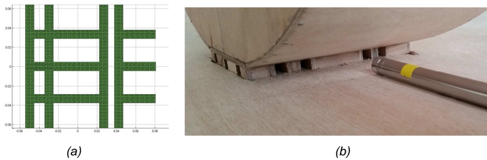
Figure 219 : (a) Optimized network; (b) Wooden optimized network between a cylinder and a plane surface
