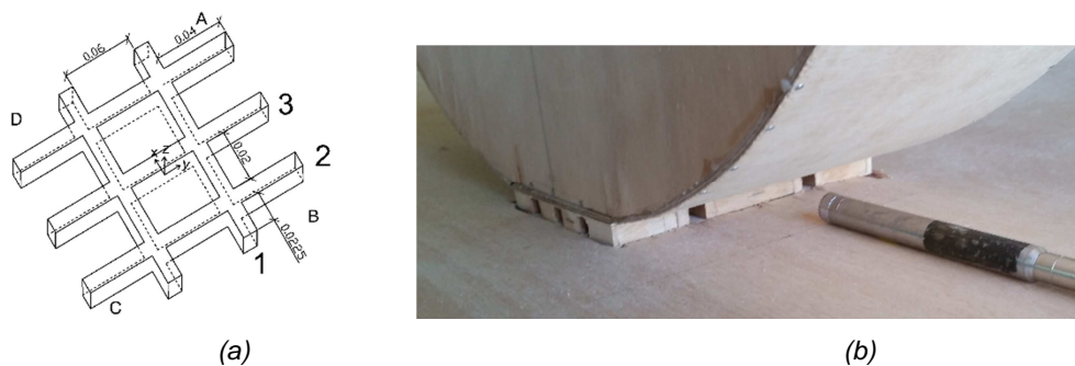
Figure 217 : (a) Network; (b) Wooden network between a cylinder and a plane surface
