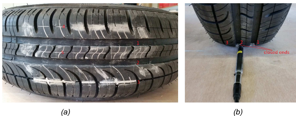
Figure 223 : (a) Tyre with an open network; (b) Tyre with a closed network
