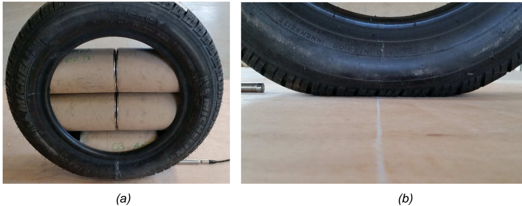
Figure 224 : (a) The load of five concrete cylinders; (b) The contact zone between the tyre and the road
