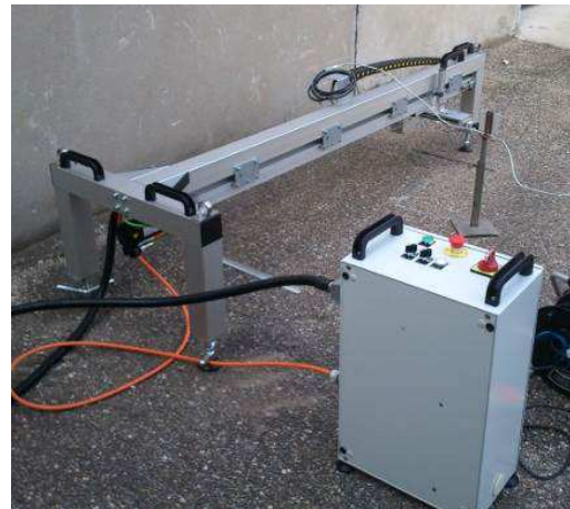
Figure 141 : New 3D texture measurement system developed at Ifsttar
