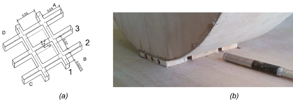
Figure 217 : (a) Network; (b) Wooden network between a cylinder and a plane surface
