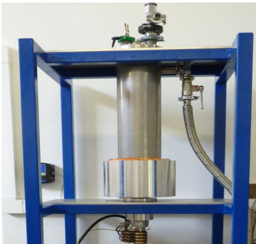
Fig.12. Photography of the superconducting motor.
