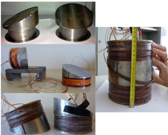
Fig. 4. Manufacture of the superconducting inductor.
