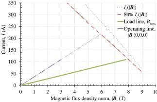
Fig. 2. Characteristic of the NbTi SC56S53 wire of SuperCon Inc. with safety margin of 20 %. Load line,  $B_{\text{max}}$  and operating line,  $|\mathbf{B}|(0,0,0)$  of the designed magnet for R = 15 cm are also shown.
