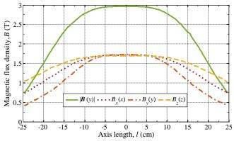
Fig. 4. Values of  $B_x(x)$ ,  $B_y(y)$ ,  $B_z(z)$ , and |B(y)| obtained with  $R_y = 15$  cm and I = 110 A. As an example, the curve labeled  $B_x(x)$  is the x-component of the magnetic field produced by the Helmholtz coil following the x-axis.
