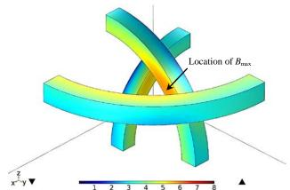
Fig. 3. Picture of the magnetic flux density norm |B| in a 1/8 model of the magnet and the location of  $B_{\text{max}}$ .
