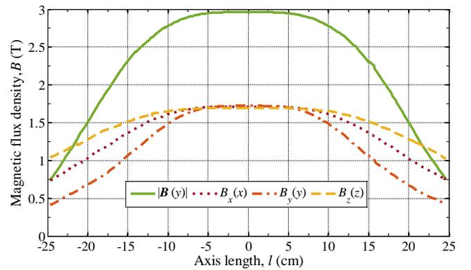
Fig. 4. Values of  $B_x(x)$ ,  $B_y(y)$ ,  $B_z(z)$ , and  $|\mathbf{B}|(y)$  obtained with  $R_y = 15$  cm and  $I = 110$  A. As an example, the curve labeled  $B_x(x)$  is the  $x$ -component of the magnetic field produced by the Helmholtz coil following the  $x$ -axis.
