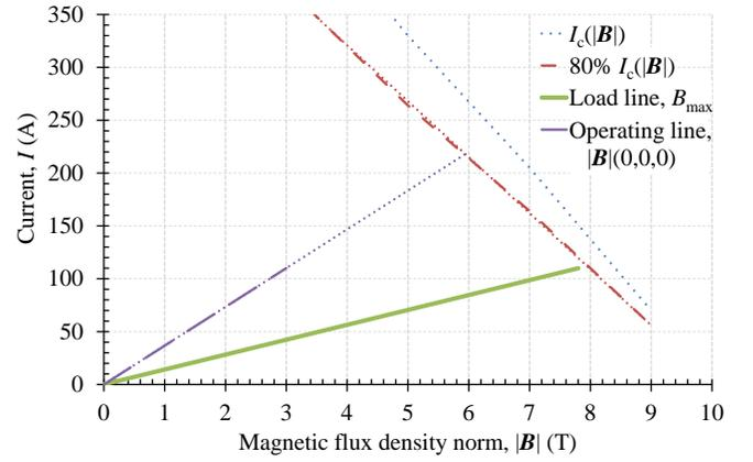
Fig. 2. Characteristic of the NbTi SC56S53 wire of SuperCon Inc. with safety margin of 20 %. Load line,  $B_{\max}$  and operating line,  $|\mathbf{B}|(0,0,0)$  of the designed magnet for  $R = 15$  cm are also shown.
