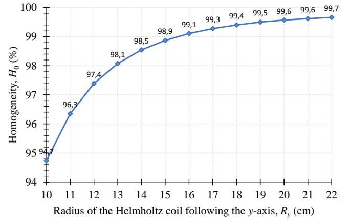
Fig. 5. Variation of the homogeneity  $H_0$  vs.  $R_y$ .
