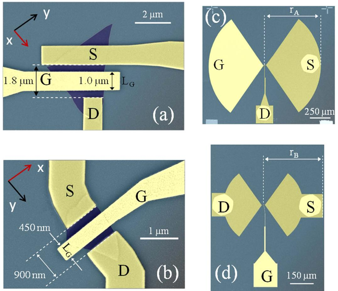
**Figure 2. Device Fabrication.** (a,b) False colors scanning electron microscope (SEM) images of the top-gated FETs in sample A (a) and sample B (b), respectively. (c,d) False colors SEM images of the patterned bow-tie antennas in sample A ( $r_A = 0.5$  mm) and sample B ( $r_B = 0.25$  mm), respectively.
