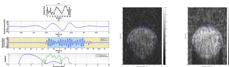
Figure 2: (a) Optimal transmitted stochastic signal  $x_{k,1}(n)$  obtained by the genetic algorithm. (b) Signal  $p(n)$  at the transducer output when  $w(n)$  was the optimal stochastic signal. (c) Corresponding radiofrequency line measured with the medium with the flaw. (d) The respective spectra. (e) Synthetic Images using the usual transmitted signal at the central frequency of the transducer  $f_c$ , and (f) the optimal stochastic signal.
