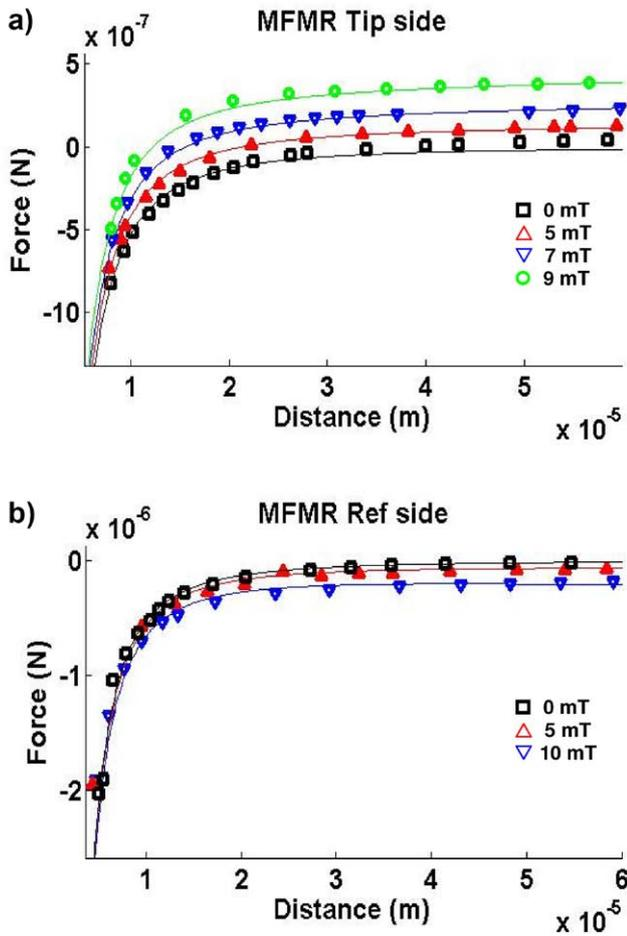
**Figure 6.** Magnetic force versus distance for MFMR probes, measured at different  $B$  values. (a) tip side configuration; (b) reflector side configuration. Solid lines: comparison with the model (equations (8)–(10)).
