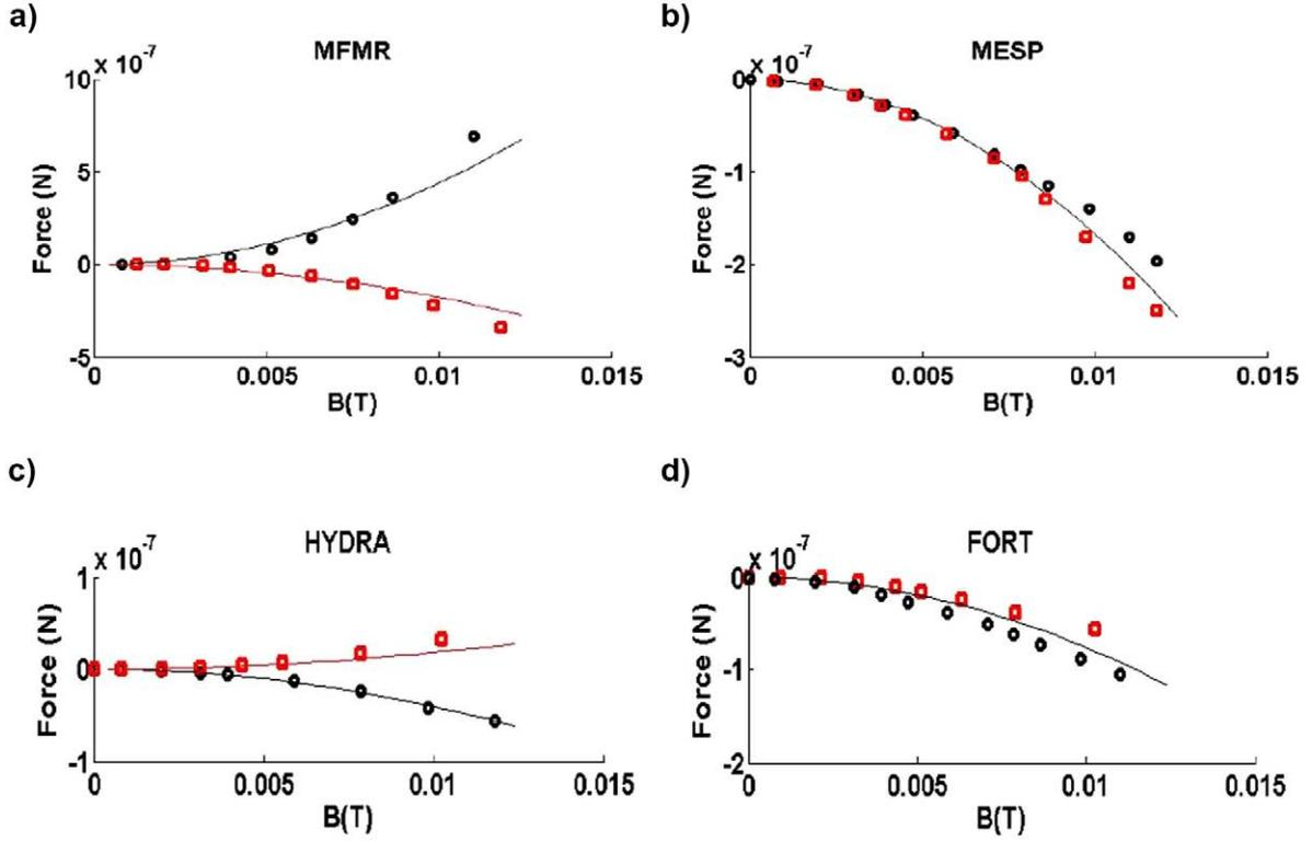
**Figure 5.** Force versus magnetic field at  $z = 100 \mu\text{m}$ . Experimental data: (○) tip side configuration; (□) reflector side configuration. MFMR (a), MESP (b), HYDRA (c) and FORT (d). Solid lines: comparison with the model (equations (8) and (9)).
