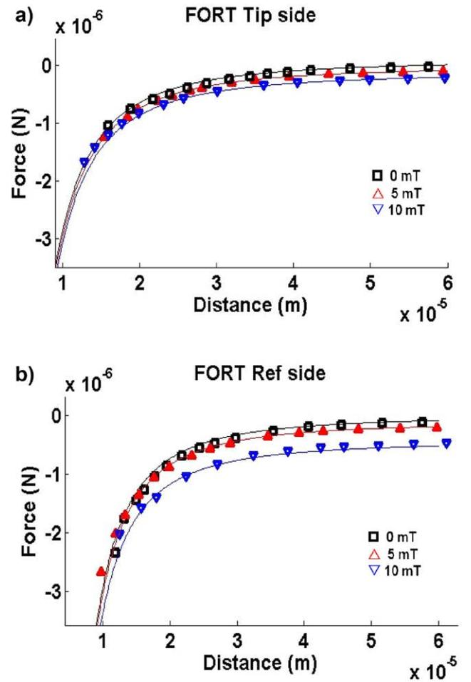
**Figure 9.** Magnetic force versus distance for FORT probes, measured at different  $B$  values. (a) tip side configuration; (b) reflector side configuration. Solid lines: comparison with the model (equations (8)–(10)).
