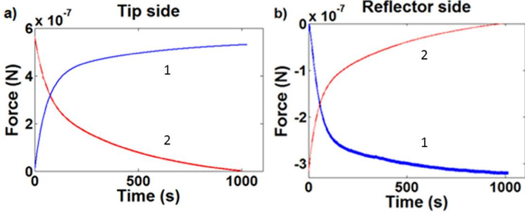
Figure 4. Typical transient regimes observed at  $z = 100 \mu\text{m}$  for MFMR cantilevers when the magnetic field ( $B = 10\text{mT}$ ) is turned on (curve 1) and then turned off (curve 2). (a) tip side configuration and (b) reflector side configuration.
