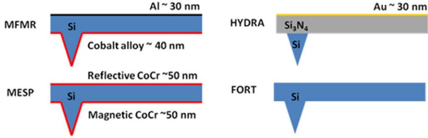
Figure 3. Commercial AFM cantilevers used in the experiments.
