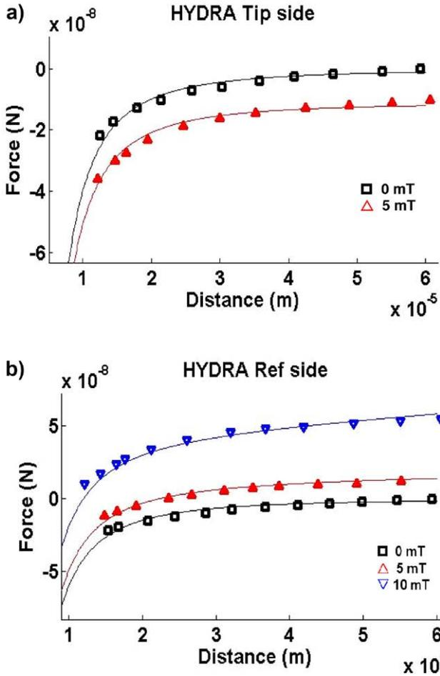
**Figure 8.** Magnetic force versus distance for HYDRA probes, measured at different  $B$  values. (a) tip side configuration; (b) reflector side configuration. Solid lines: comparison with the model (equations (8)–(10)).
