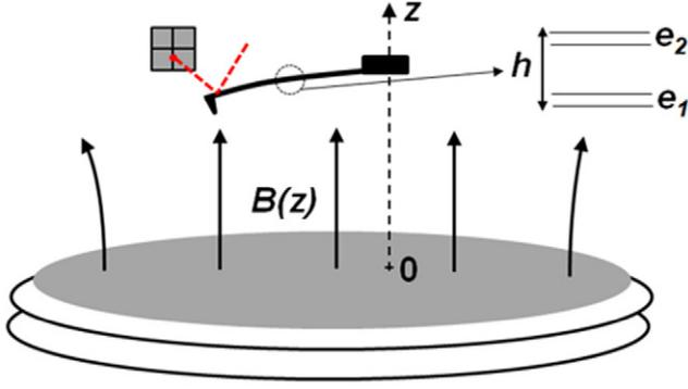
**Figure 1.** Schematic representation of the experimental set-up. An AFM probe is placed in an external magnetic field produced by a large coil with iron core. For a three-layer cantilever of total thickness  $h$ ,  $e_1$  is the thickness of the coating on the tip side and  $e_2$  on the reflector side.
