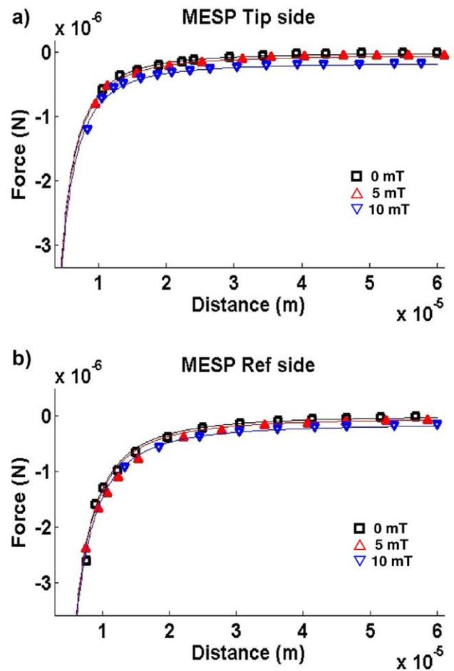
**Figure 7.** Magnetic force versus distance for MESP probes, measured at different  $B$  values. (a) tip side configuration; (b) reflector side configuration. Solid lines: comparison with the model (equations (8)–(10)).
