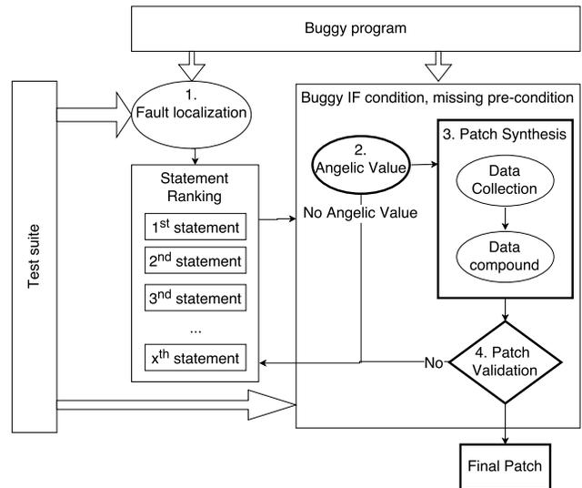
**Figure 3: Overview of the Nopol repair system.**
