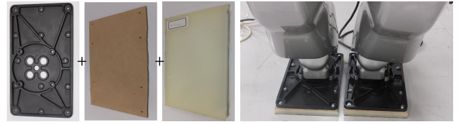
Fig. 7: Photo of HRP-2's feet with flexible soles
