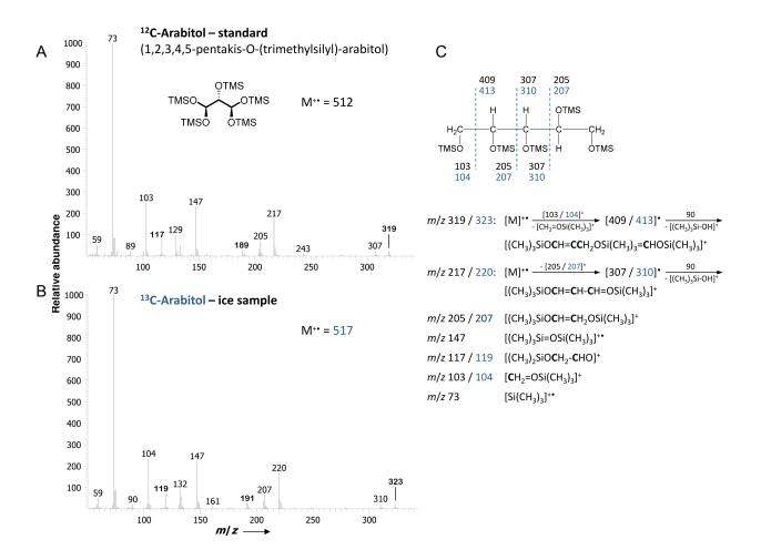
**Fig. S4. Mass spectra of the <sup>12</sup>C-arabitol standard (A) and the <sup>13</sup>C-arabitol ice sample (B).** The arabitol fragmentation pattern is indicated (C) by representing the individual mass shifts for each fragment of the <sup>12</sup>C standard (black) and the <sup>13</sup>C sample (blue).
