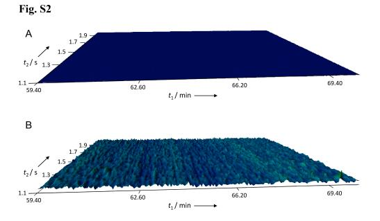
**Fig. S2. Analytical blank.** A: Representative enantioselective GC×GC–TOFMS chromatogram of the blank sample submitted to the entire analytical protocol. Atomic mass units 206 and 294 (×5) were selected for the above representation and the primary and secondary temperature program was identical to Figure S1. B: Reduced *z*-scaling (*z*-axis = 5,000) illustrates the absence of monosaccharides and other related compounds in the blank sample.
