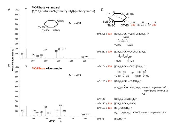
Fig. S3. Mass spectra of the <sup>12</sup>C-ribose standard (A) and the <sup>13</sup>C-ribose (B) identified in the pre-cometary ice sample. The ribose fragmentation pattern is indicated (C) by representing the individual mass shifts for each fragment of the <sup>12</sup>C standard (black) and the <sup>13</sup>C sample (red).
