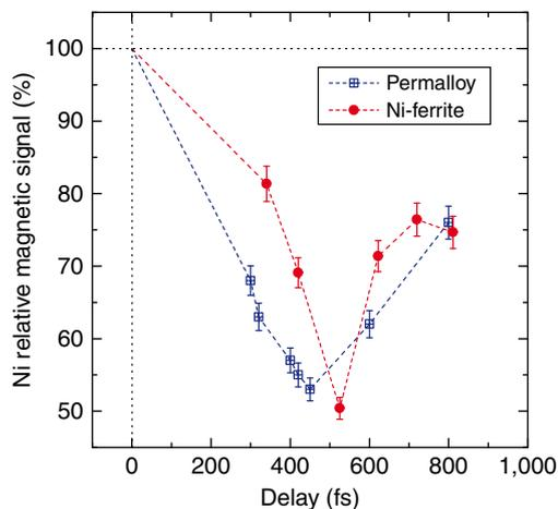
**Figure 5 | Time-dependent magnetic signal.** Ni demagnetization in the permalloy (blue squares) and the Ni-ferrite (red circles) samples at several delays  $\Delta t$  between probe and pump pulses ( $F = 10 \text{ mJ cm}^{-2}$ ). Vertical error bars represent s.d. (see Methods). The maximum fluctuation in the pump-probe delay over the measurement duration ( $\pm 5$  fs, see Methods) is smaller than the point width. Lines are a guide to the eye.
