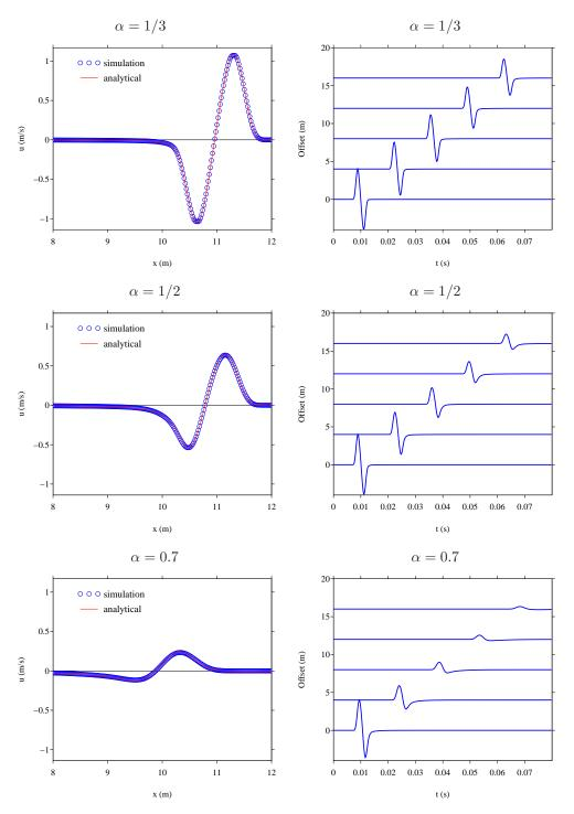
Fig. 6. Test 1: time-domain simulations of linear fractional advection, for various orders of the fractional order  $\alpha$ . Left row: snapshots of the numerical and exact solutions. Right row: simulated seismograms.
