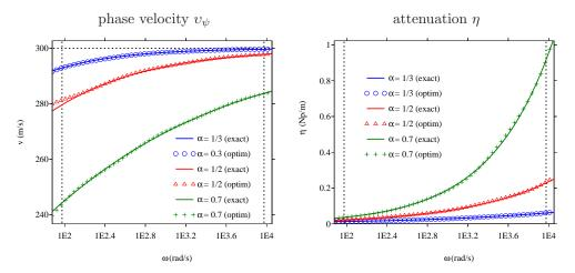
Fig. 2. Comparison between the dispersion curves of the fractional model (2.1) and of the diffusive model (3.2). The parameters are a=300 m/s, b=0,  $\varepsilon=1$  s<sup> $\alpha-1$ </sup>,  $\alpha=1/3$ , 1/2 and 0.7, and L=4 diffusive variables. The quadrature coefficients are obtained with the optimization procedure. The horizontal dotted line denotes the sound velocity a. The vertical dotted lines denote the range of optimization.
