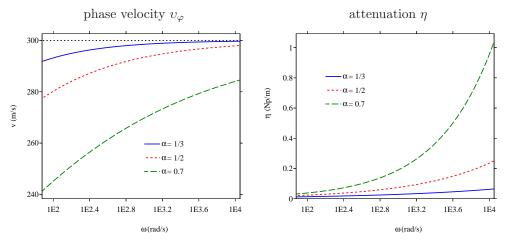
Fig. 1. Dispersion curves deduced from (2.9) in the linear regime (b = 0), with a = 300 m/s,  $\varepsilon = 1$  s<sup> $\alpha$ -1</sup> and various values of  $\alpha$ : 1/3, 1/2 and 0.7. The horizontal dotted line in the phase velocity denotes the sound speed a.
