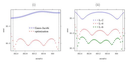
Fig. 3. Error of model  $\left|\frac{\tilde{\chi}(\omega)}{\chi(\omega)}-1\right|$  deduced from (2.8) and (3.7). The parameters are a=300 m/s,  $\varepsilon=1$  s<sup>-1/2</sup> and  $\alpha=0.5$ . Left row (i): Gauss-Jacobi and optimization methods are compared, for L=4 diffusive variables. Right row (ii): optimization is used, and various values L are considered. The vertical dotted lines denote the range of optimization.
