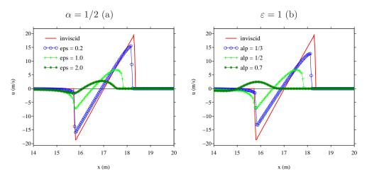
FIG. 8. Test 3: snapshots of the numerical solutions at t=0.06 s. Nonlinear advection and fractional attenuation are considered. (a)  $\alpha=1/2$ , and various values of  $\varepsilon$ . (b)  $\varepsilon=1$ , and various values of  $\alpha$ .
