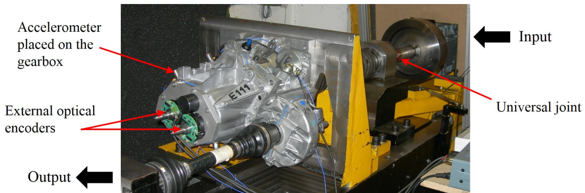
Figure 3: Instrumented gearbox on the LaMCoS test bench.
