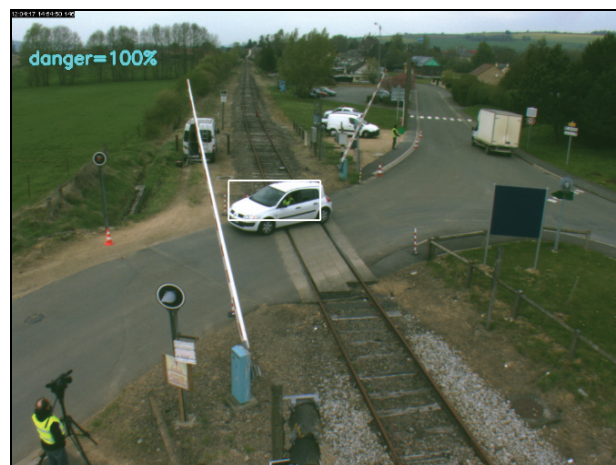
Fig. 6 Automatic detection of a car stopped on a level crossing.
