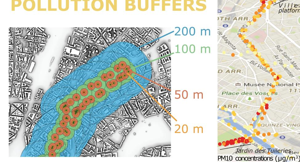
Each point represents a mean of particle concentration measurements during 30 seconds. We made different size of buffer (20 m, 50 m, 100 m and 200 m) for each point to combine the PM concentrations average and the urban morphological parameters.
