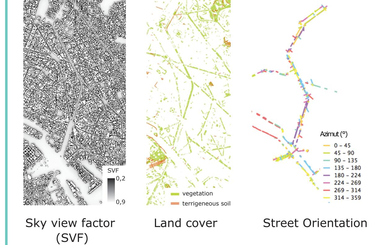
We rasterized vector layers (street orientation and land cover) to calculate the mean/proportion of SVF, street orientation and different types of land to each pollution data buffer with the raster calculator.
