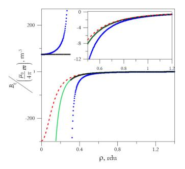
**Figure 4.**  $B_z(\rho, \vartheta = \pi/2)$  dependences for a uniformly magnetised sphere of radius R = 0.3 rdu (circles, grey online), a circular current loop of radius R = 0.3 rdu, (diamonds, blue online) and a pair of fictitious magnetic charges, d = 0.3 rdu apart, (dashed, red online) compared do that of the point dipole (continuous, green online). The inset: shows a zoom in the behaviour of  $B_z$  at larger distances.
