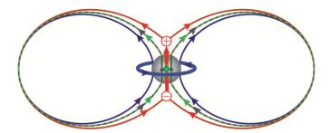
**Figure 5.** Magnetic field lines for different dipole models scaled in rdu. The external line (red online) corresponds to a pair of magnetic charges d = 0.75 apart. The intermediate dashed (green online) and continuous (grey online) lines refer to a point dipole and uniformly magnetised sphere of radius R = 0.20, respectively. The internal line (blue online) is due to a current loop of radius R = 0.40. All the lines merge at the maximal distance  $r_{\text{max}} = 2.0$ .
