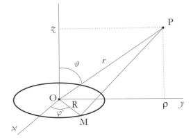
Figure 2. Magnetic dipole modelled by an Ampérian current.
