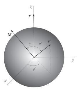
Figure 1. Magnetic dipole modelled by a uniformly magnetised sphere.
