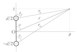
Figure 3. Magnetic dipole modelled by an assembly of two 'magnetic charges'.
