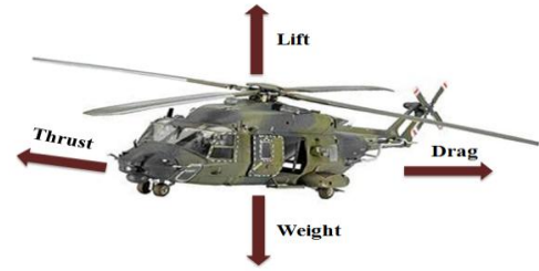
Figure 1. The Four Forces Applied to a Helicopter
