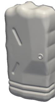
FIGURE 13: Photographies of the baffled oil pan under study. The measures of the pressures and the acoustic velocities have been done using a pU probe. The oil pan is excited by a shaker fed with white noise.
