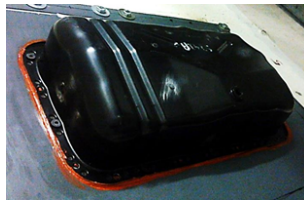
FIGURE 13: Photographies of the baffled oil pan under study. The measures of the pressures and the acoustic velocities have been done using a pU probe. The oil pan is excited by a shaker fed with white noise.
