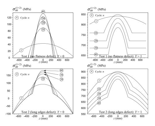
Fig. 3:  $\sigma_{\theta\theta}^{(1+2)}$  profile along the axial direction
