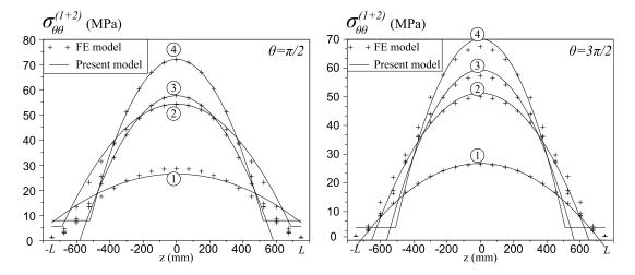
Fig. 2: FEM validation at Y = 1 with Abaqus
