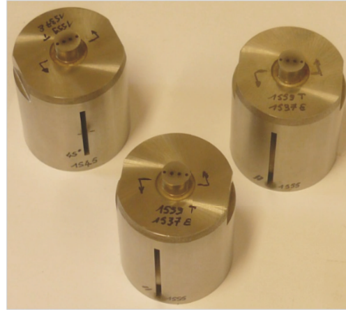
Figure 6: Plug design and the manufactured plugs with their 4 aligned holes for Optical Fibers insertion
