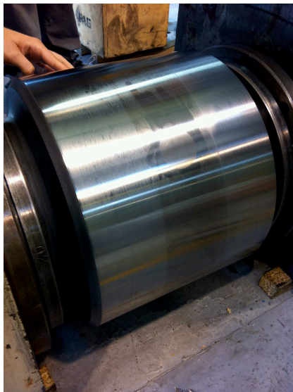
(a) Work roll with its instrumented plug
