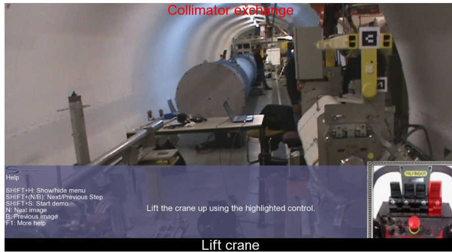
Fig. 5. Application layout. The HUD menu is displayed over the AR view.
