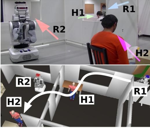
Fig. 4. The real robot example. The bottom picture the 3D model, with the object path as a white arrow. The solution involves successively R1, H1, R2, H2, and the object is handed over through the windows, minimizing H1 efforts, and brought directly to H2 so he doesn't have to move.
