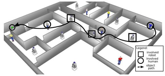
Fig. 3. The big rooms example, with a solution represented by the black arrow. Seven agent out of sixteen are part of the plan. This plan tries to minimize delivery time. Other solutions avoiding humans would use only robots and pass by the room at the bottom of the image.
