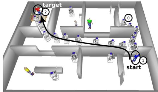
Fig. 1. An example in an environment where agents are separated into two navigable zones linked by windows and counters. The blue human is in possession of an object needed by the red one. The solution found by our algorithm is: robot 0 navigates to the blue human, takes the object through a handover over the counter, and then navigates to the red human and gives it to him.
