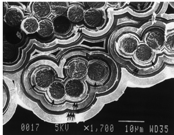
FIGURE 17.13 Morphology of self-healing matrix inside a yarn from Reference 1.
