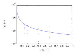
**Figure 4**: Fiber bundle lifetime vs. partial oxygen pressure, at  $T = 500^{\circ}C$  and  $\sigma = 1,000 MPa$ : predicted lifetime of the bundle's critical fiber (*i.e.* the fiber with 5 % failure probability) vs. [4]'s experimental data
