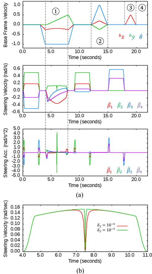
Fig. 3 Simulation results of the proposed numeric treatment; (a) base frame velocity trajectory  $b\dot{\xi}$  of the first four benchmark tests (top), the corresponding steer joint rate commands (middle) and steer joint acceleration (limit of  $5 \text{ rad/s}^2$ ), (b) the effect on the second steer joint rate  $\hat{\beta}_2$  passing kinematic singularity along with the steer rate variation with  $\delta_2$ .
