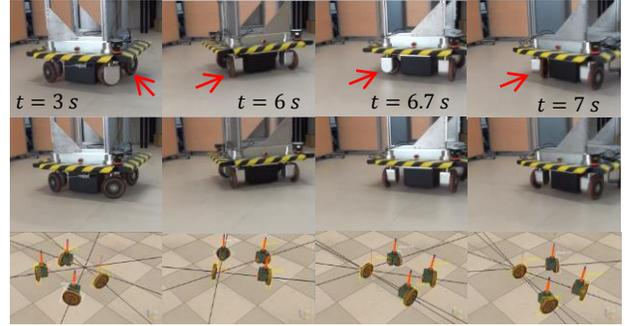
Fig. 4 Snapshots of the two experiments (test 1, with singular joint indicated by the red arrow). Top: embedded controller, Middle: developed model. Bottom: v-rep<sup>1</sup> simulation showing the ICR position.
