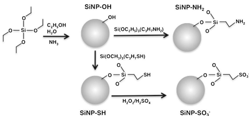
**Scheme 1** Preparation of silica nanoparticles (SiNP-OH) and their surface modification by amine (SiNP-NH<sub>2</sub>), thiol (SiNP-SH) and sulfonate (SiNP-SO<sub>3</sub><sup>-</sup>) groups
