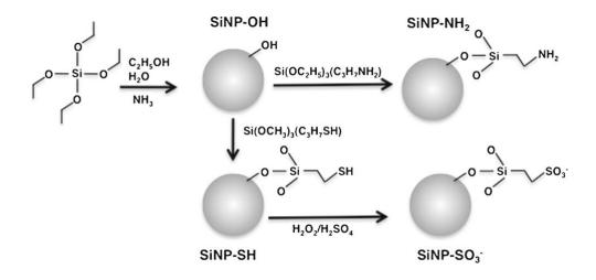
Scheme 1 Preparation of silica nanoparticles (SiNP-OH) and their surface modification by amine (SiNP-NH<sub>2</sub>), thiol (SiNP-SH) and sulfonate (SiNP-SO<sub>3</sub>-) groups
