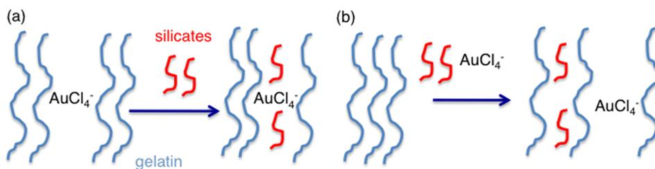
FIG. 3. Schematic illustration of the impact of experimental procedure on the localization of gold species upon silicification: (a) gelatin-stabilized  $\text{AuCl}_4^-$  remain trapped within the hybrid particles; (b) unstabilized  $\text{AuCl}_4^-$  are expelled from silicate proximity and migrate to the gelatin phase.
