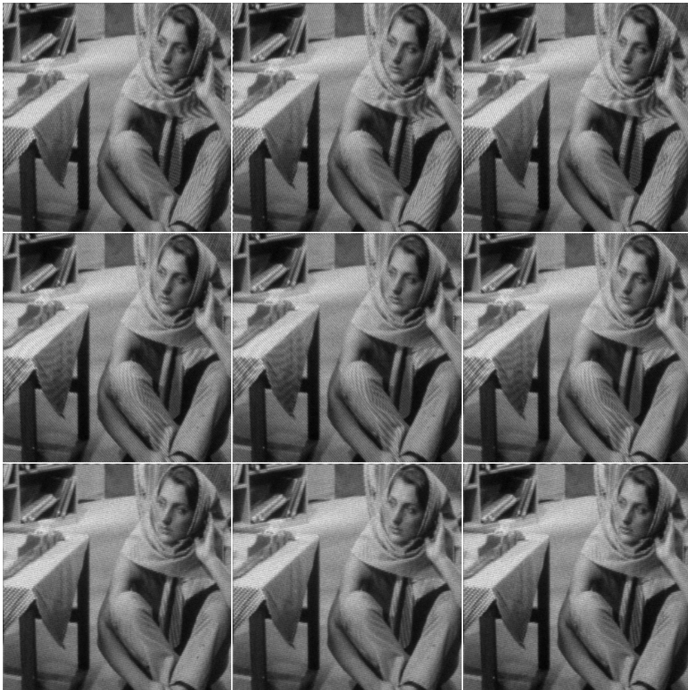
Figure 6: Set of nine 256 \times 256 simulated SIM images from the standard "barbara" test image. We can observe that the modulations pattern produces a Moiré effect revealing the underlying high frequencies.
