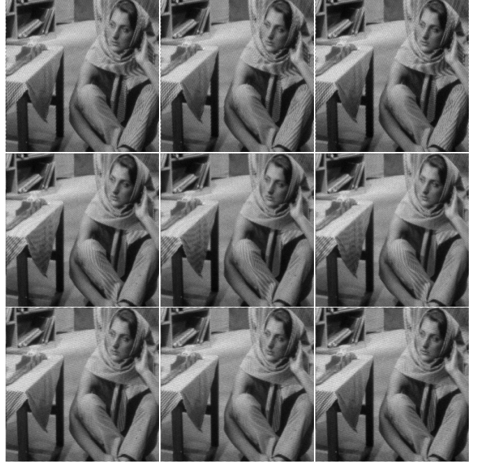
Fig. 5. Set of nine 256 \times 256 simulated SIM images from the standard “barbara” test image. We can observe that the modulations pattern produces a Moiré effect revealing the underlying high frequencies.
