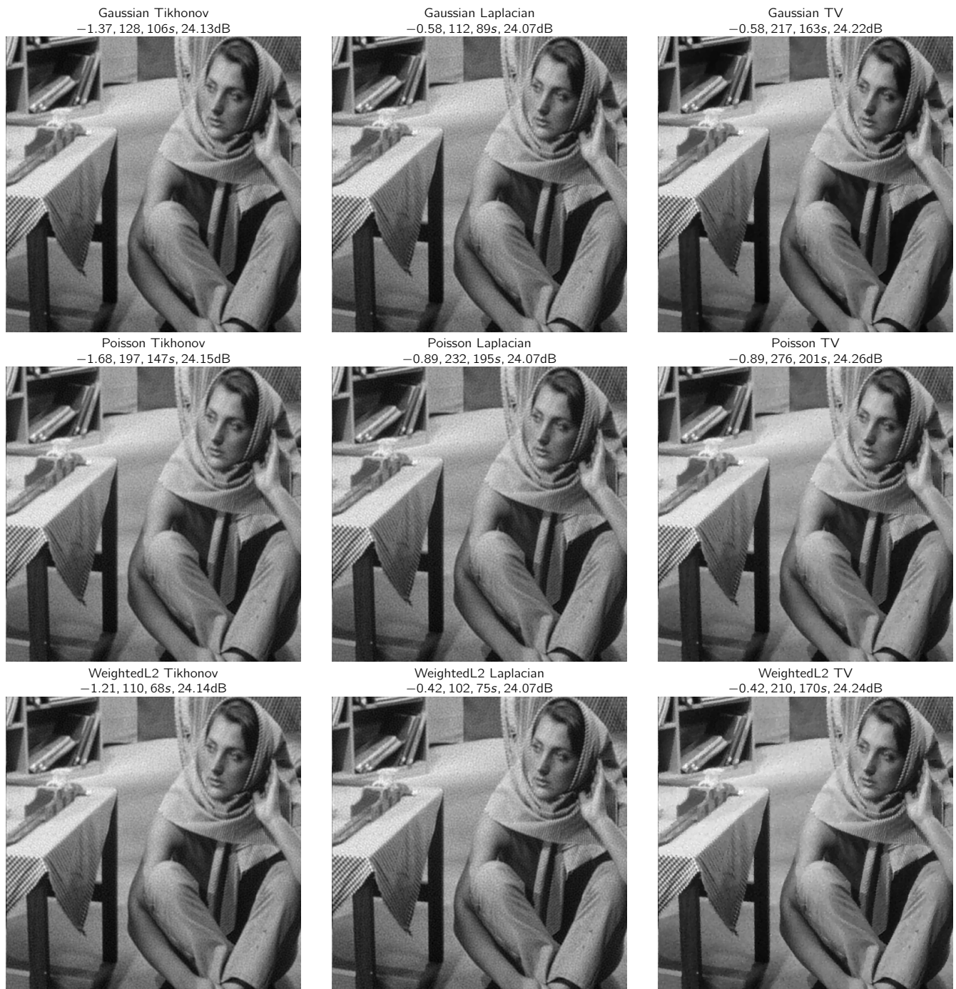
Fig. 8. Comparison of 18 functionals on the “barbara” standard test images. For each case, the regularization parameter (in a \log_{10} basis), the number of iterations and the computation times and the PSNR are indicated. The displayed image and values correspond to the maximum PSNR on a range of regularization parameters with in the interval [\log_{10}(-2), \log_{10}(1)] .
