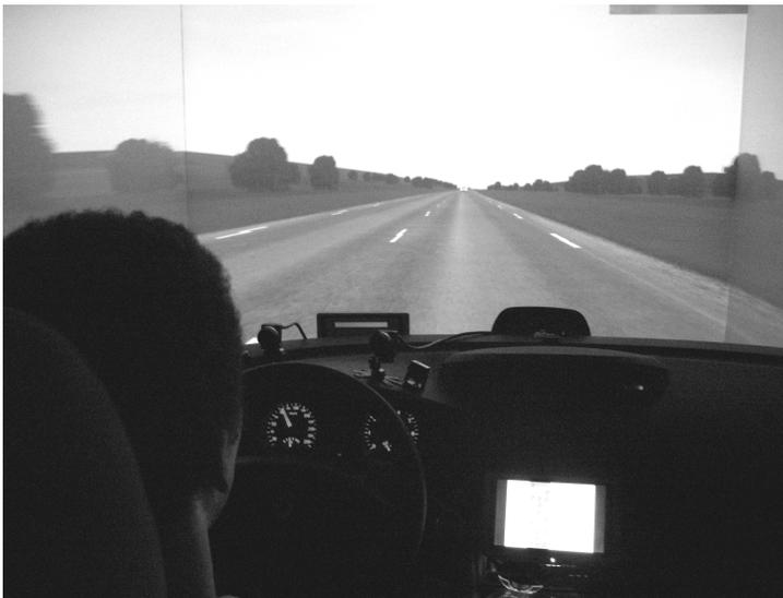
**Figure 1. Illustration of simulator setup, showing the FCW system displaying an alarm (red bar) and the secondary task interface (on the bottom right)**
