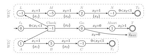
**Fig. 14.** Reach( $\leq 1$ ): Simulation to decrement counter  $C_1$
