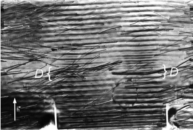
Figure 12. Transmission topograph of the SAW propagating on a large ST-cut delay line operating at 9.507840 MHz.
