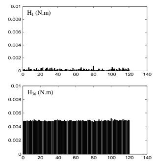
Fig.5. Magnitudes of the harmonics 1 (top) and 36 (bottom) for 120 realizations of the torque when I=0.5 A.
