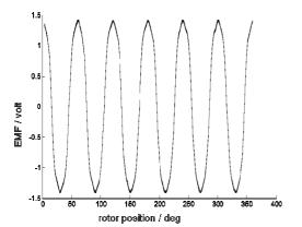
Fig.4. 120 realizations of the EMF when taking into account the eccentricity and I=0.5 A  $\,$
