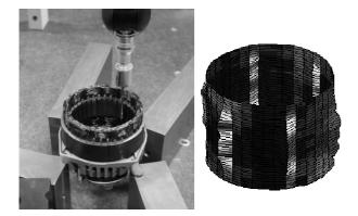
Fig. 1. Measurement of the inner surface of the stator (left) and 3D representation of the deformation of this surface from the measured points (right).
