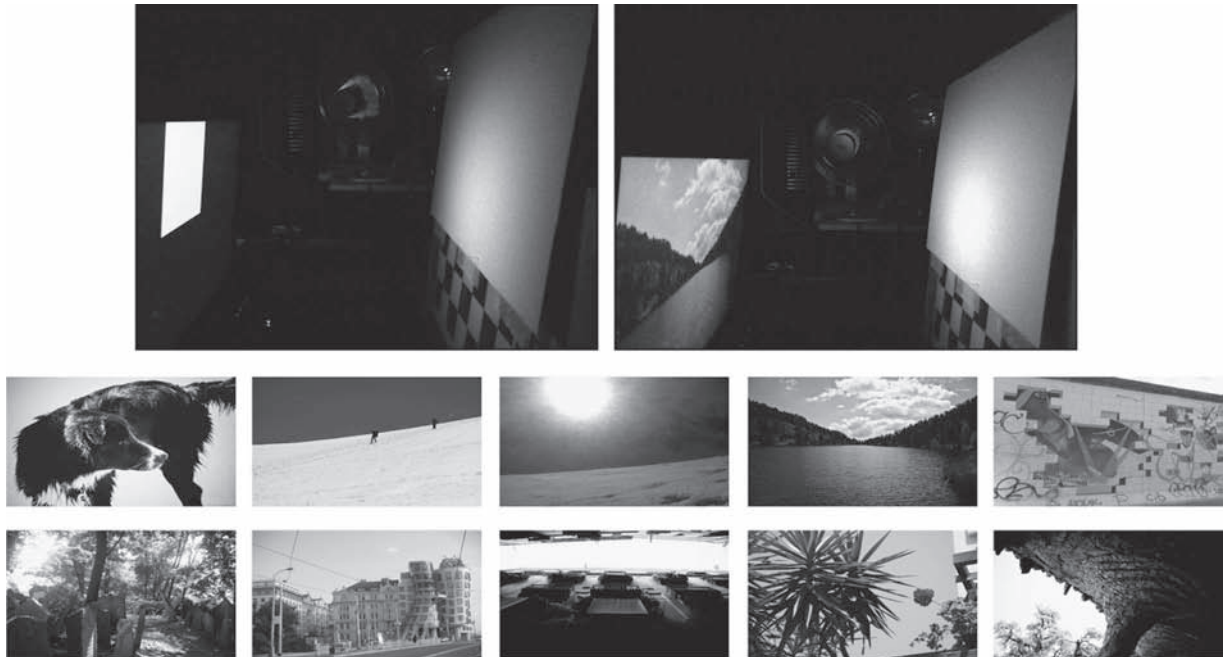
Fig. 5. Experimental setup. Top: a screen (laptop HP EliteBook8570w) displaying a rectangular pattern (left) or a graylevel image (right) in front of a white planar sheet of paper. Bottom: real images used in the experiments. All images are of size 1600 \times 900 (screen resolution).
