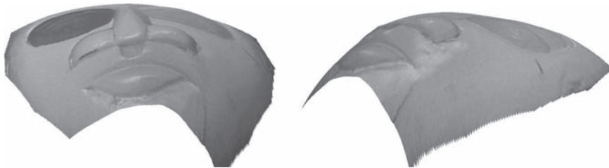
Fig. 17. 3D-reconstruction by photometric stereo, using the standard directional approximation [3,5,7]. Neglecting the extended behavior of the screen creates a large-scale bias, preventing realistic applications.
