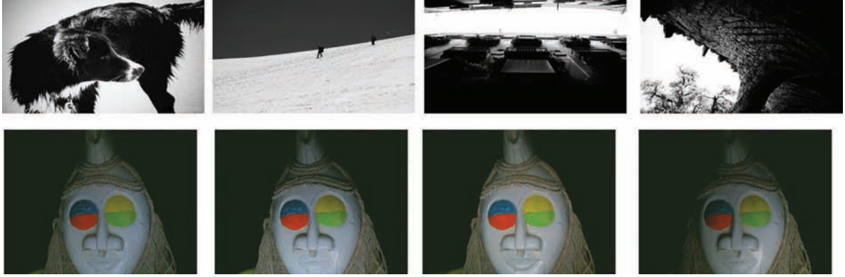
Fig. 13. As a person watches a slideshow of images (first row, we show 4 out of 40 images), pictures are recorded (second row). The pictures displayed on the screen serving as light sources, we employ the photometric stereo approach to recover the geometry and photometry of the scene.
