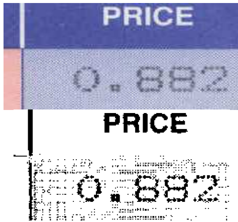
Figure 6 : The succession of operations to segment color images containing inverted and not inverted texts.
